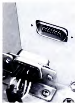
All leads to the deck go through this plug-in connector. There is nothing to disconnect to remove the deck.
