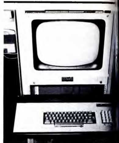
Figure 2 This is an operator's eye of the keyboard and CRT. The board layout includes an auxiliary numeric pad on the right which controls cursor positioning and scrolling through the computer memory. This feature allows the operator directly examine and edit the memory contents. The Dataphone on the left is used to tie the system into Market for access to ARB data. The CRT is used by the operator at all times except when finished hardcopy is produced.
