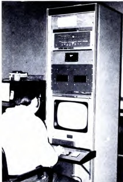
Figure 1 The author is shown at the operating position of the computer system. From top to bottom the equipment is as follows: switching panel, Altair 8800 computer, mini floppy disc drive, digital cassette drives, video monitor, and keyboard. The system power supply (not in photo) is in the bottom of the rack.
