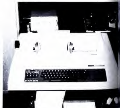
Figure 3 This is the DECwriter printer used for hardcopy for finished logs. It also allows the system to handle special forms and mail labels when the computer is used in an automatic typewriter mode.
